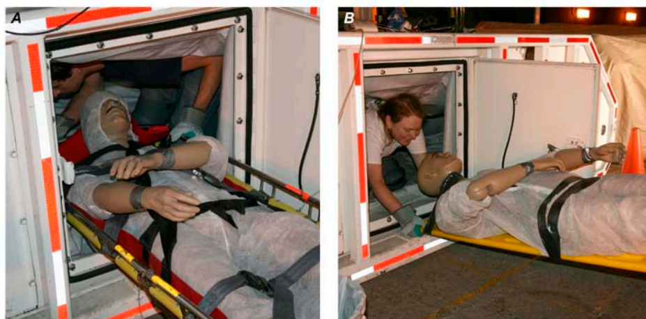
Figure 7: Moving the A) splint stretcher and B) full-length hard backboard stretcher into the inflatable RA airlock.
