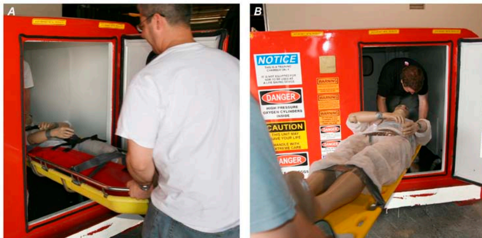
Figure 6: Moving the A) splint stretcher and B) full-length hard backboard stretcher into the rigid steel RA airlock.
