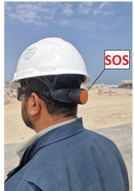
Photo 1: Smart helmets include valuable features such as built-in sensors and a panic (SOS) button.
