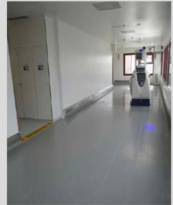
Photos 5 (left) and 6 (right): Automated/automatic guided vehicles (AGVs) are typically fitted with many controls such as lasers, cameras and other sensor devices to identify and mitigate collision exposures. They can also be programmed to maintain a specified path and reduce speed or stop if specific parameters are not maintained.
