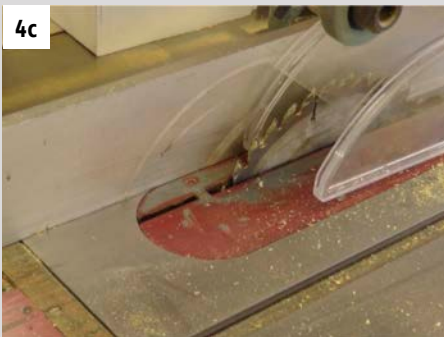
Figure 4c: No anti-kickback or splitter devices in- stalled.
