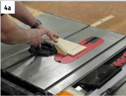
Figure 4a: SawStop saw without blade guard.
