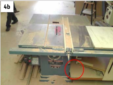
Figure 4b: Table saw with no blade guard in- stalled.
