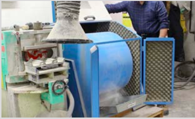
Photo 1: Los Angeles abrasion machine used to study the quality of coarse aggregate. The machine generates a great amount of visible aggregate dust despite the use of a dust extractor.
