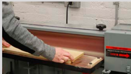
Photo 5: Edge sander used to sand down the edges of wooden material. The machine generates a great amount of wood dust, but a local exhaust ventilation system is often used when in operation.
