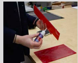
Photo 13: Process of gluing acrylic plates using acrylic or super glue. This process hardly generates any fumes, but on rare occasions an adhesive spray may be used.
