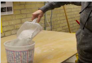
Photo 10: Plaster-casting powder being poured into pail before use. The process generates plaster dust, and a local exhaust ventilation system is used.
