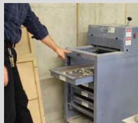
Photo 11: Coarse aggregate shaker used to sieve aggregate stone or rock to different levels of fineness. The machine barely generates aggregate dust, as it is covered when in use.
