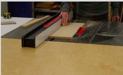
Photo 4: Table saw used to cut pieces of wood and acrylic plastics. The machine generates a great amount of dust, but a local exhaust ventilation system is often used when in operation.
