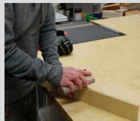
Photo 12: Piece of wood being sanded using a manual hand sander. This process hardly generates any wood dust.
