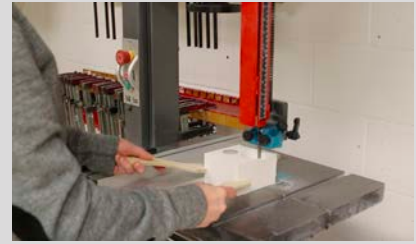
Photo 3: Band saw used to cut pieces of wood, plaster molds and acrylic plastics. The machine generates a great amount of dust, but a local exhaust ventilation system is often used when in operation.
