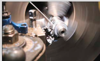
Photo 7: Lathe used to shape metals by rotating it against a stationary cutting tool. The machine generates smoke when the cutting tool gets too hot or fumes if a coolant is used as well. Metal chips created by this machine are dusted off, but no local exhaust ventilation system is used for the airborne contaminants.
