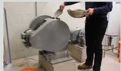
Photo 9: Jaw crusher used to crush aggregate stone or rock. The machine generates aggregate that falls into a tray. Respirators are used and a local exhaust ventilation system is turned on when machine is operating.
