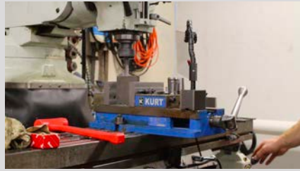
Photo 2: Milling machine used to create grooves, holes and irregular surfaces on metals. The machine generates a great amount of metal dust, and no local exhaust ventilation system is used.
