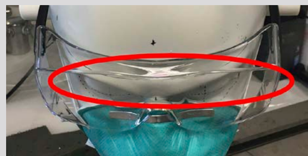
FIGURE 13 GAP BETWEEN EYE PROTECTOR & WEARER'S FOREHEAD
