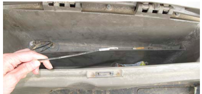
Photo 1: Heavy equipment rental with no operator's manual. The manual should have been attached to the wire shown. The operator cannot safely operate the equipment until one is obtained. This machine had an important piece of safety hardware, an item called the swing lock pin, improperly placed by the rental company.
