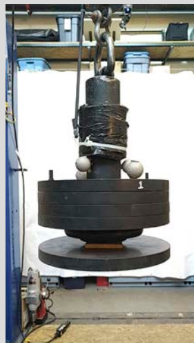
(Clockwise from top) Photo 1: NIOSH drop structure located in High Bay Laboratory. Photo 2: The advanced dynamic anthropomorphic mannequin (ADAM) was equipped with a full body harness. Photo 3: Modified 234-lb drop weight.
