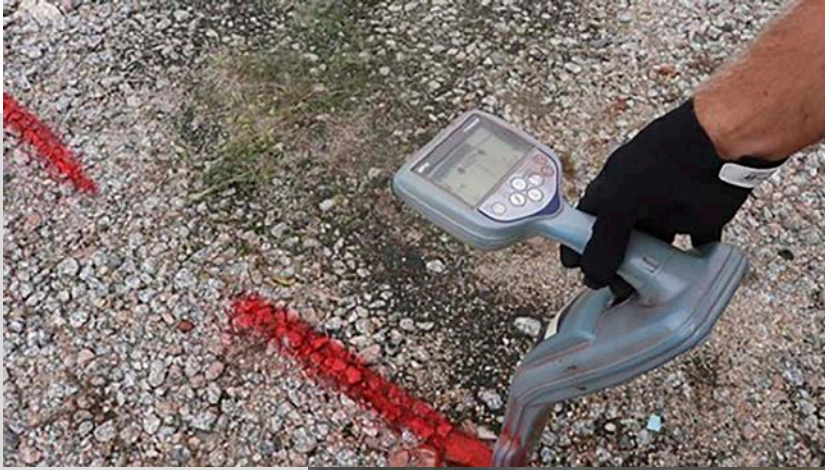
Photo 1 (above): A cable locating device. These devices use geospatial technology and rely on electromagnetic sensors or radio frequency and ground-penetrating radar to map components below the surface.
