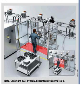
Imagine the improvement in safety and productivity when a worker can walk into a machine and the control-reliable sensors and controls put the machine in a safe mode for performing a given task. Such a system, shown in Figure 3, looks simple and is sometimes referred to as "passive safeguarding."
